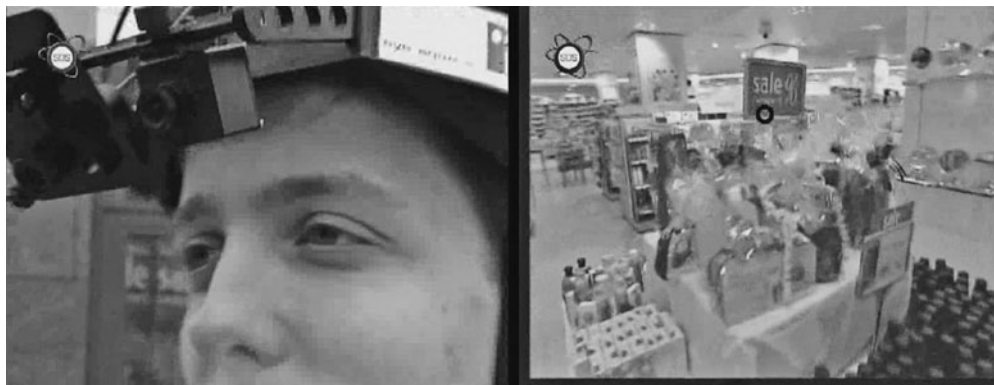
Fig. 6.1. Eyetracker used in a shopping mall for evaluation purposes. Copyright eyesquare.
