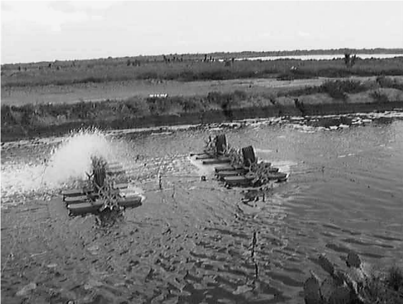
Fig. 15.9. Mechanical aeration in discharge canal at Harlingen Shrimp Farms, Inc.
