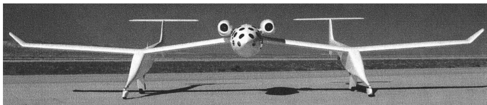
Fig. 2.3. View of Scaled Composites' White Knight , intended to be used to provide a high-altitude airborne launch of their manned sub-orbital spacecraft, SpaceShip One (courtesy: Scaled Composites).
