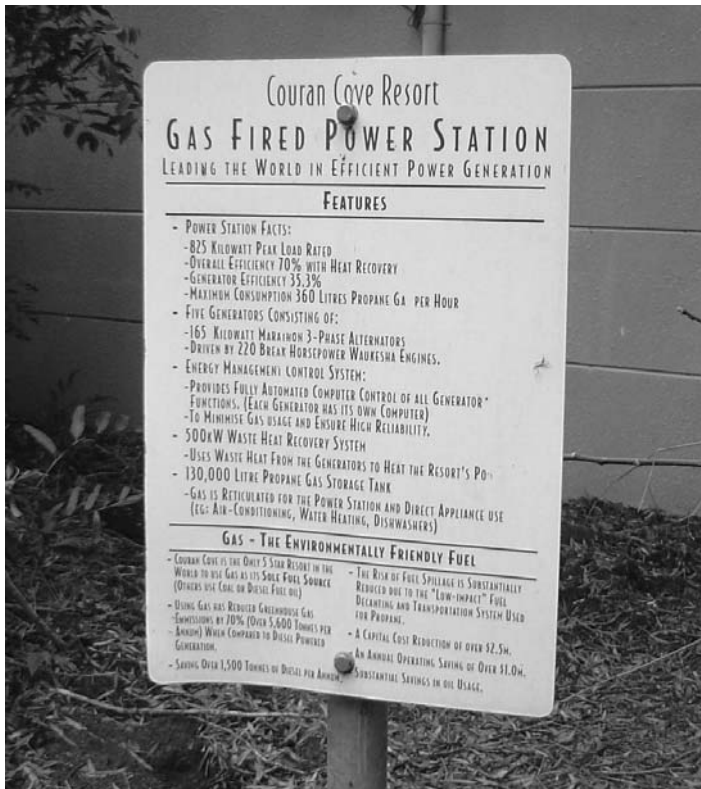
Fig. 8.3. Features of gas-fired power station, Couran Cove, Stradbroke Island, Queensland, Australia (photograph courtesy of C. Cater).
