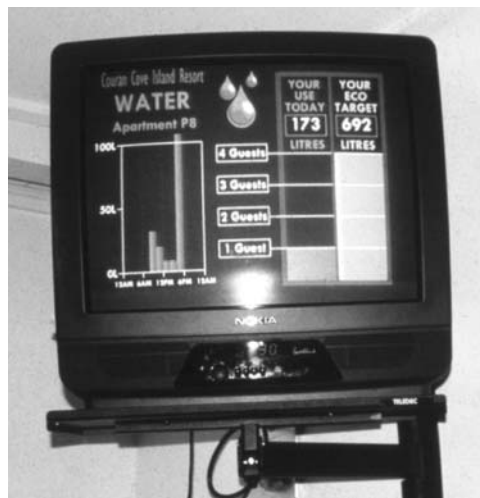
Fig. 8.4. Guest water consumption displayed on TV monitor, Couran Cove, Stradbroke Island, Queensland, Australia (photograph courtesy of E. Cater).
